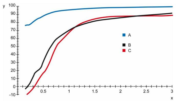
Y = Efficiency (%), X = Particle size (μm) A = NOM filter, B = Centrifugal filter A, C = Centrifugal filter B Efficiency of NOM main filter compared to typical centrifugal filters, tested with DOP.
